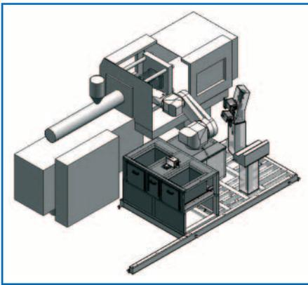
Robot with injection molding machine in clean room Class 6/7
