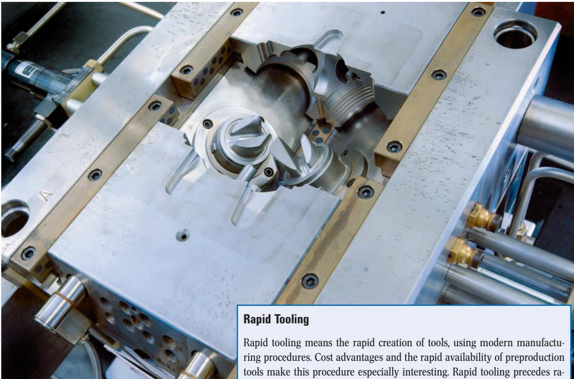
The right product solution is the one thing, the appropriate tools for the manufacture of the product is the other. Rapid tooling, rapid prototyping and Moldflow all belong to the 1+1 of the plastics engineer.
