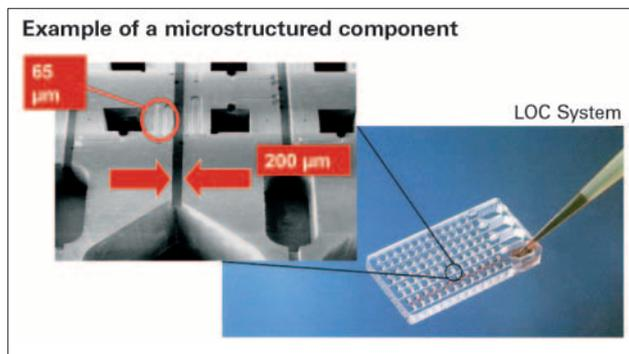
The health sector is going through the same changes as the computer world. Small and more exact solutions: Left: Close-up of the lab-on-a-chip. Right: Lab-on-a-chip for the blood analysis. (Illustrations: STEAG microParts GmbH, Germany)
